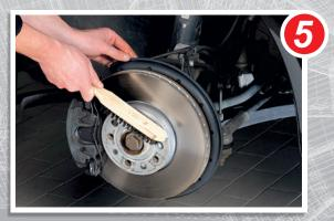
5. Perfect cleanliness It is imperative that the hub is free of rust and/or corrosion residue.
